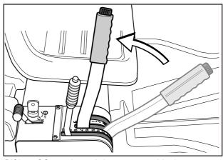
Lifting of the cutting unit (transport position)
